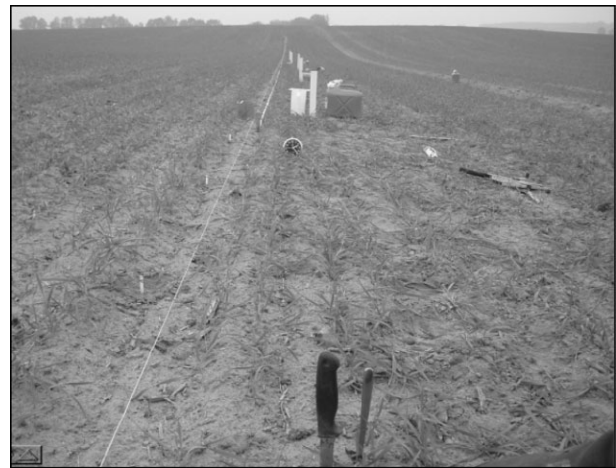
Figure 1: Transect in tillage direction with 101 locations, 1 m apart, between two winter wheat rows; October 2006 (Photo: Brandt).
