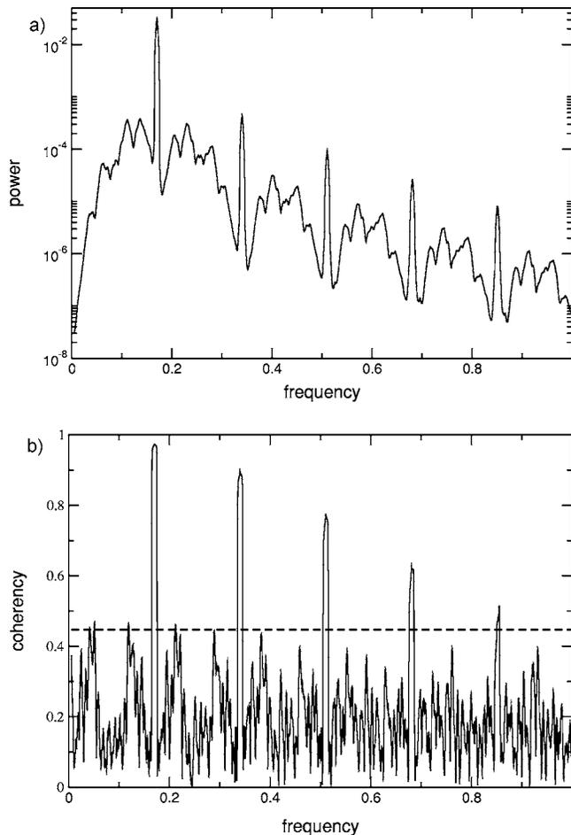
FIG. 1. (a) Power spectrum of the  $x$  component of the Rössler system at the vicinity of the main oscillating frequency. (b) Coherency of two independent, identical Rössler systems. The coherency at frequencies of approximately 0.17 and its multiples are lying above the 5% level of significance (dashed line).
