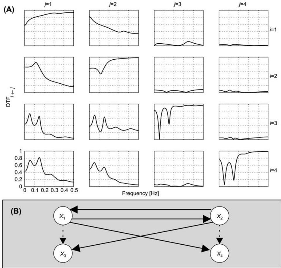
**Figure 4** (A) Directed transfer function for the VAR model considered. The auto-directed transfer functions  $\delta_{i \leftarrow i}$  are shown on the diagonal. The directions of the simulated interactions are revealed correctly by directed transfer function analysis. Nevertheless, two indirect interactions are inferred from process  $X_1$  to  $X_3$  and process  $X_2$  to  $X_4$ . This is indicated by the dashed arrows in the graph in (B).
