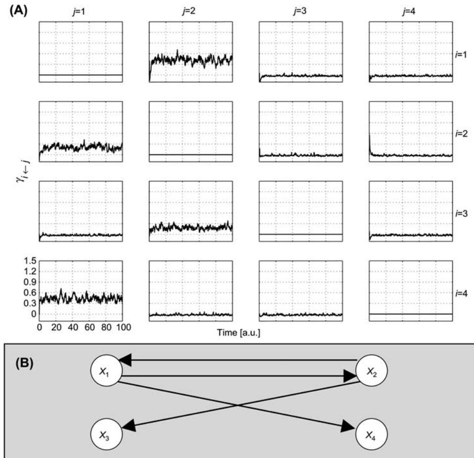
**Figure 3** (A) Granger causality index for the VAR model and (B) the resulting directed graph. The simulated interrelation structure is reproduced correctly by non-zero values of the Granger causality index. a.u., arbitrary unit.
