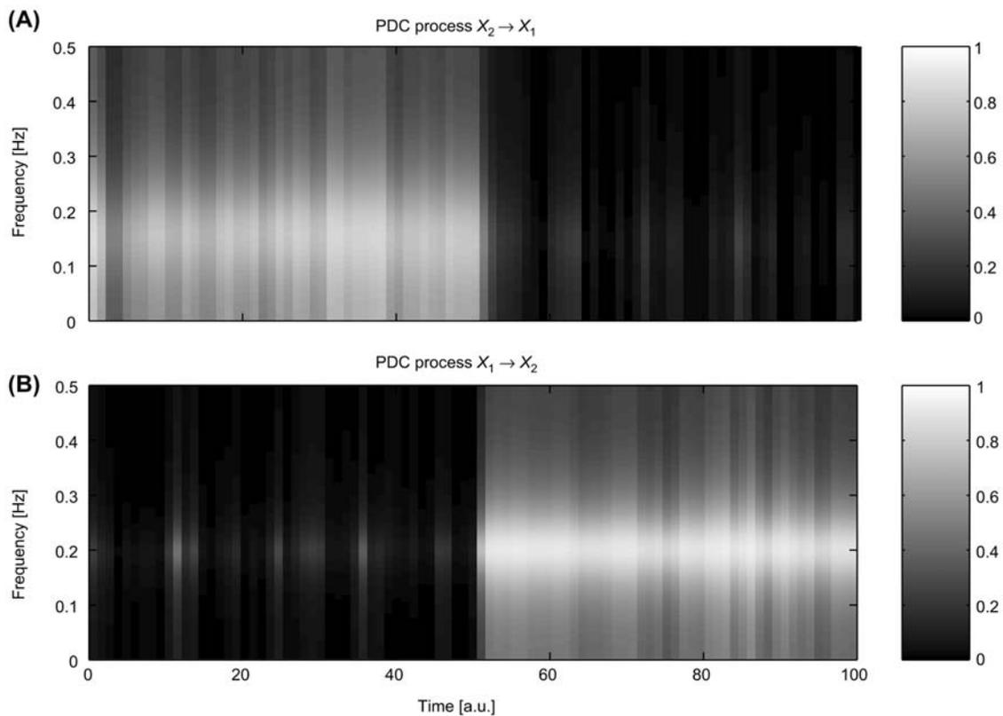
**Figure 6** Application of time-resolved partial directed coherence. The transition in the interaction structure between processes  $X_1$  and  $X_2$  is detected correctly. a.u., arbitrary unit.
