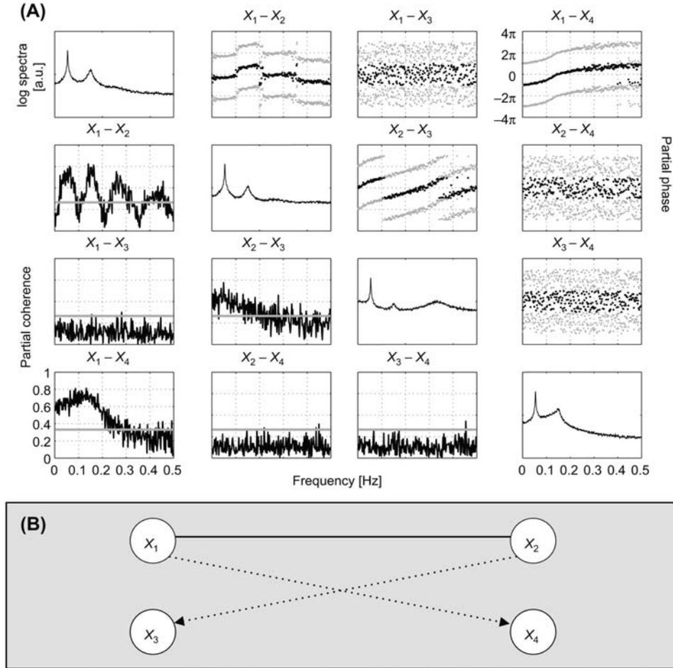
**Figure 2** (A) Partial coherence and corresponding phase spectra. Auto-spectra are shown on the diagonal, with partial coherence spectra below the diagonal and partial phase spectra above the diagonal. Differentiation between direct and indirect influences is possible. However, the bidirectional interaction between  $X_1$  and  $X_2$  is not traceable by evaluating the phase spectra. (B) Graph summarizing the results.
